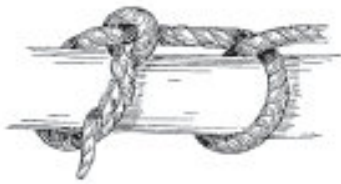
FIG. 39.—Timber hitch and half-hitch.
