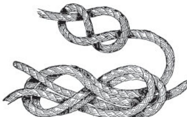
FIG. 25.—Double figure-eight knot (tying).
