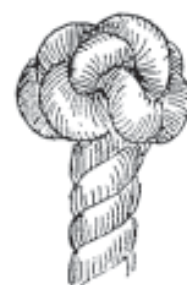
FIG. 125.—Wall crowned (complete).
