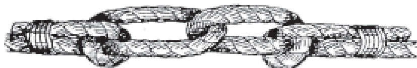
FIG. 29.—Half-hitch and seizing.
