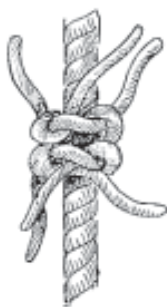
FIG. 118.—Shroud knot (making).
