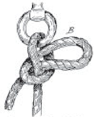
FIG. 30.—Lark's head with toggle (A).
