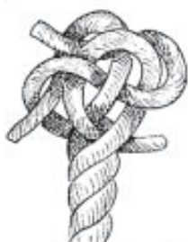
FIG. 121 A.—Making double crown.
