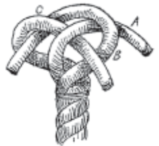
FIG. 111.—Single crown (making).
