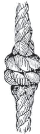
FIG. 117.—Shroud knot (complete).
