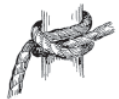
FIG. 36 B.—Clove hitch (complete).
