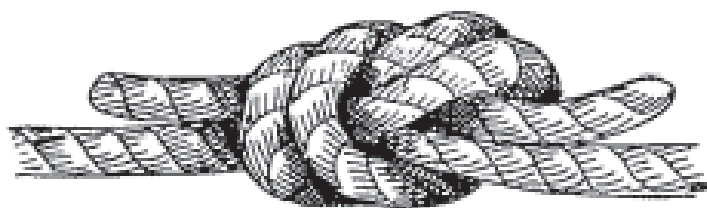
FIG. 19.—Ordinary knot (finished).
