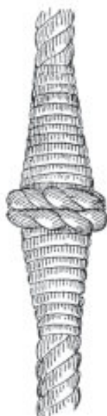
FIG. 120.—French shroud knot (complete).
