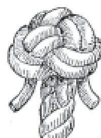
FIG. 126.—Double wall and crown.
