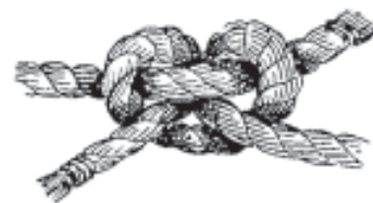
FIG. 14.—Slipped square knot.
