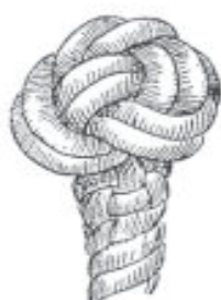
FIG. 127.—Double wall and crown (complete).
