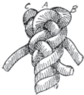
FIG. 112.—Single crown tucked (making).
