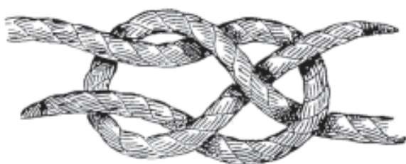
FIG. 28.—Simple hitch (hawser).
