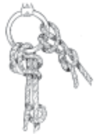
FIG. 56.—Larks' heads and running noose.
